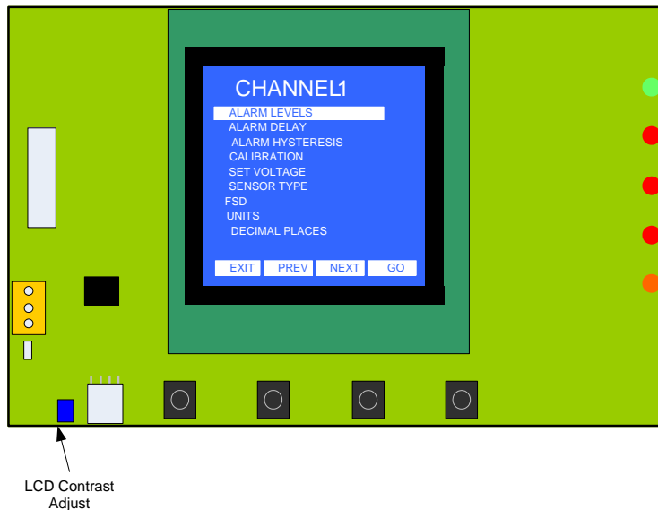
Figure 4: LC-8 Display Contrast Adjustment
