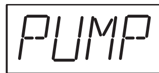
PUMP – Pump Failure
