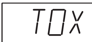
TOX – Electrochemical Sensor Failure
