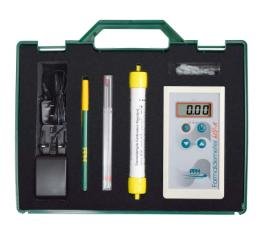
Portable handheld detectors available for monitoring O<sub>2</sub>, CO, CH<sub>4</sub>, and combustibles.
